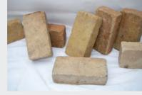
Fire-proof bricks are used as refractories to line glass furnaces, kilns, and incinerators. Waste fire-proof bricks generated by the demolishing of such facilities and periodic repair work are collected and carefully sorted. Recyclable items are reused as paving materials and fire-proof bricks.
